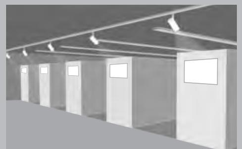
**Track lighting systems** provide flexibility in different room situations. Luminaires or spotlights can be inserted at any point on the track using an adapter, providing light to wherever it is needed.
