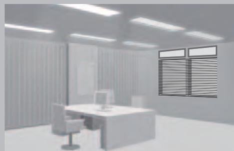
**Daylight systems** channel light into the room and protect against glare at the same time. Movable or stationary systems can be installed on the inside or outside of façades, or integrated into the façade or roof surface.
