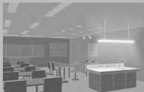
**Pendant luminaires** are mounted at a distance below the ceiling and serve as design elements in a room. They provide direct/indirect light distribution and come in a wide variety of designs.
