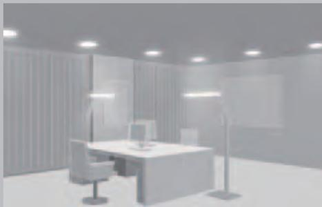
**Surface-mounted luminaires** are attached to ceilings or walls. Downlights can be surface-mounted or recessed luminaires.
