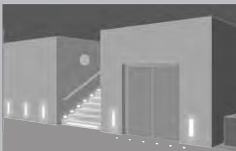
**Recessed wall and floor luminaires** are often used to highlight danger zones.
