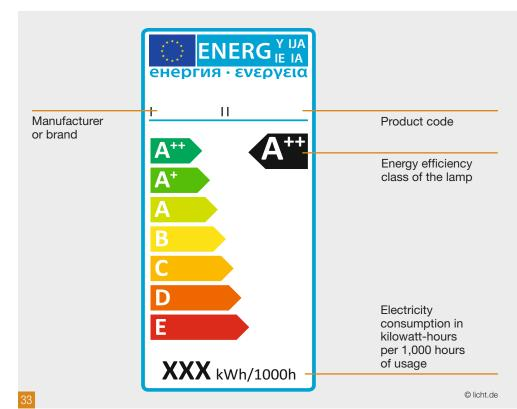
[33] The energy label for lamps (as of September 2013) shows details of a lamp's energy efficiency class. LEDs and efficient energy-saving and fluorescent lamps are particularly economical in their use of electricity.
