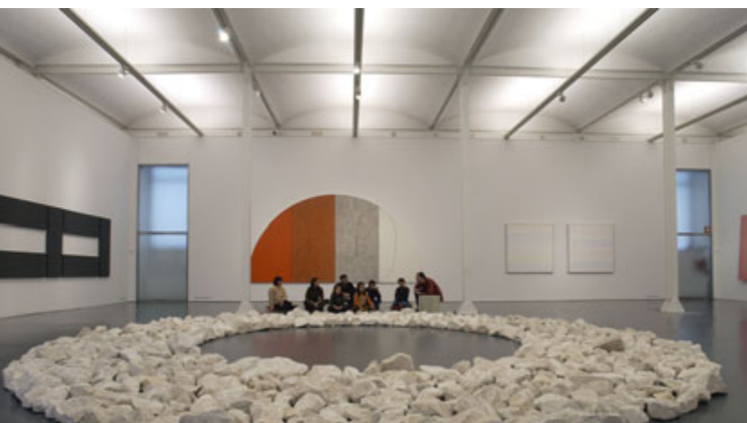
Photo 4: Luminous ceilings are particularly suitable for painting galleries. The cove lighting provides additional brightness.
