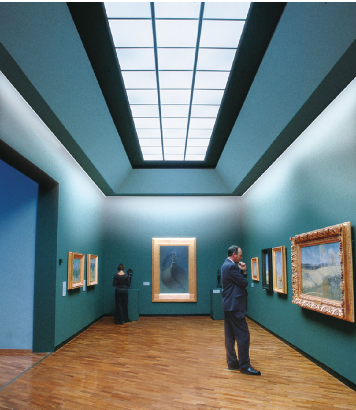
Photo 4: Luminous ceilings are particularly suitable for painting galleries. The cove lighting provides additional brightness.
