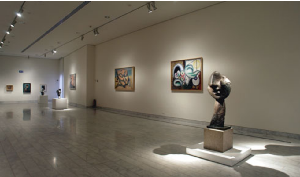
Fig. 4: Indirect and direct components produce diffuse and directional lighting respectively
