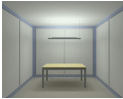
Light for working: pendant luminaire for tubular fluorescent lamp with direct/indirect light distribution
